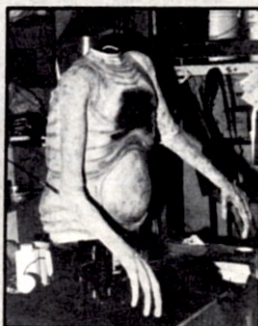
Far Left: Robert Short attaches the latex arms to the plastic "heart-light" chest. Above: Don Pennington and Lucy Seaman adjust the brace that supported E.T.'s mechanical head. Note the thin dowels protruding from the elbows, a muppet-like arm movement. Cables leading out the back of the chest were attached to air bladders, which made the heart pulsate. Left: The completed chest, painted to match the foam latex versions.
